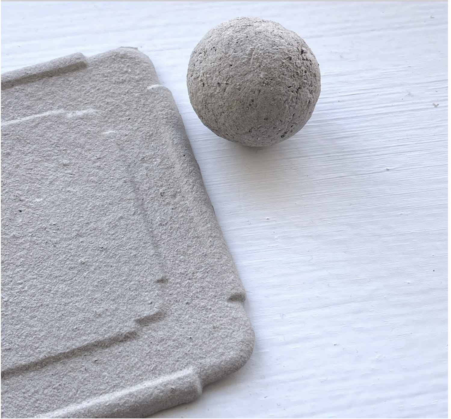
Agar and Wood-ash Based "Concrete"
