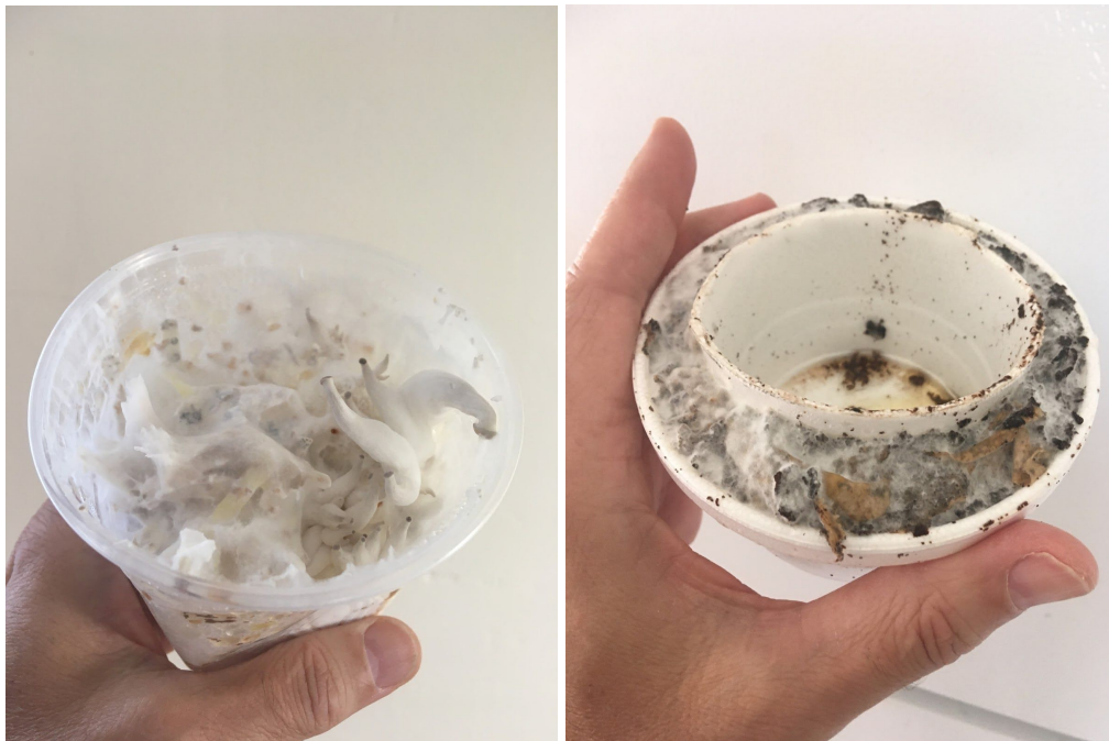
(LEFT: used coffee filters showing mycelium growth)(RIGHT: filled mold made from styrofoam containers)
